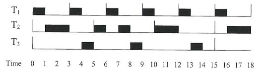
For example, in the above figure, tasks  $T_1$ ,  $T_2$ ,  $T_3$  with execution time 1, 2, 3 and periods 3, 5, 15 respectively are feasible using the preemptive EDF scheduler.  $T_1$ ,  $T_2$ , and  $T_3$  first finish execution at time 1, 3, and 14 respectively. The whole schedule repeats at 15.  $T_2$  is preempted by  $T_1$  at time 6 and resume at time 7,  $T_3$  is preempted by  $T_2$  at time 5 and resume at time 8, preempted again by task  $T_1$  at time 9 and resume at time 13.
